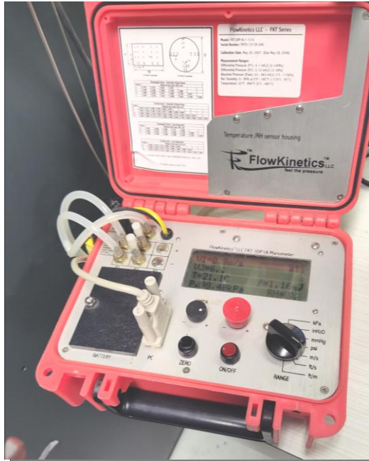
Figure 2: The FlowKinetics Manometer and its density measurement on the day of the experiment ( 1.16 \text{ kg/m}^3 )
